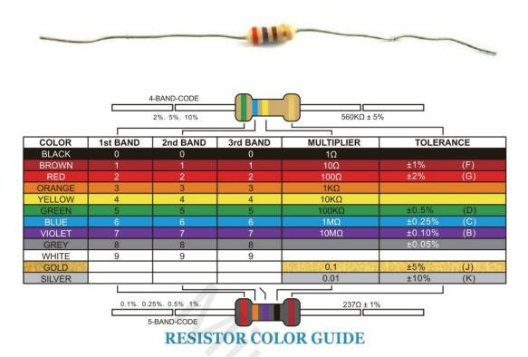
As the name suggests, resistors resist the flow of electricity. The higher the value of the resistor, the more it resists and the less electrical current will flow through it.
