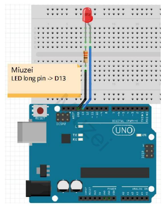
Note : The longest LED of the pin is connected to the digital signal port 13(D13).
