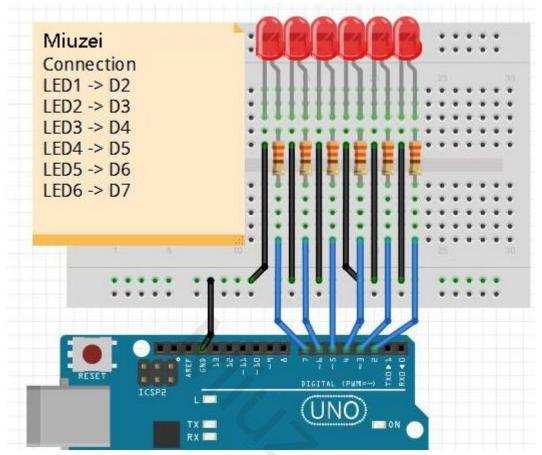
Note: The longest LED of the pin is connected to the digital signal port \*(D\*).
