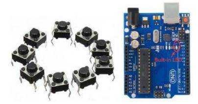
Pushbuttons or switches connect two points in a circuit when you press them. This example turns on the built-in LED on pin 13 when you press the button.
