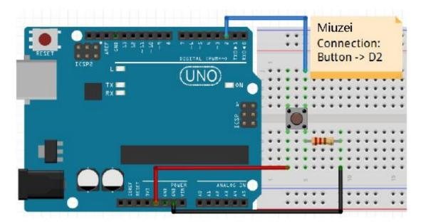
Connect three wires to the board. The first two, red and black, connect to the two long vertical rows on the side of the breadboard to provide access to the 5 volt supply and ground. The third wire goes from digital pin 2 to one leg of the pushbutton. That same leg of the button connects through a pull-down resistor (here 10K ohm) to ground. The other leg of the button connects to the 5 volt supply.
