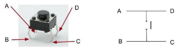
Actually, there are only really two electrical connections, as inside the switch package pins B and C are connected together, as are A and D.
