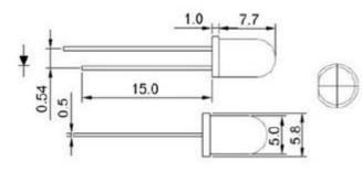
★ Pin definition It is the definition of LED pin Long pin -> + (VCC) Short pin -> - (GND)
