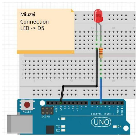
Note : An LED connected to digital output pin 5 (D5) through a 220 ohm resistor.
