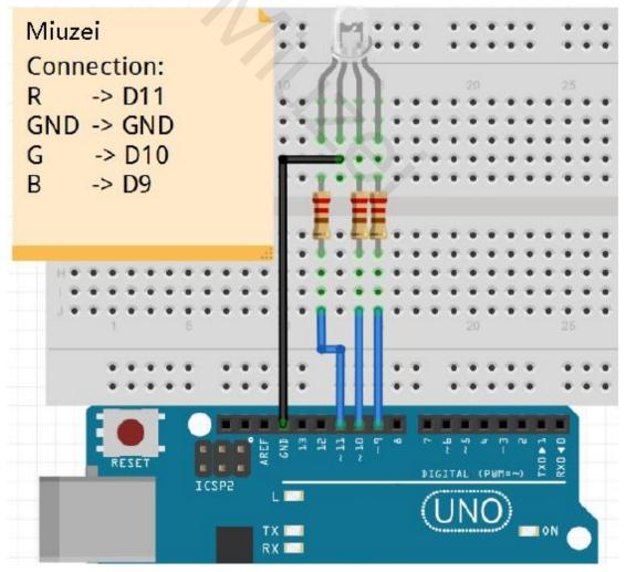
Note: The longest pin of the RGB LED is connected to the GND.
