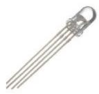
In this lesson, you will learn how to use a RGB (Red Green Blue) LED with an Arduino. You will use the analogWrite function of Arduino to control the color of the LED.
