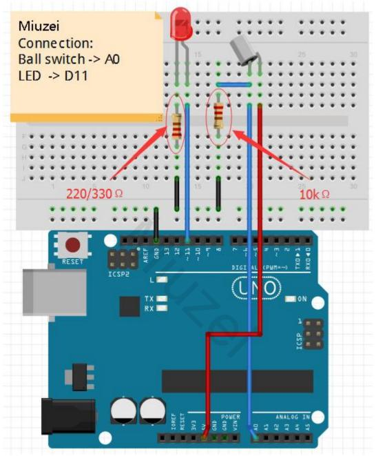
Note: The longest LED of the pin is connected to the digital signal port 11 (D11). Ball switch's pin is not divided into positive and negative polarity.
